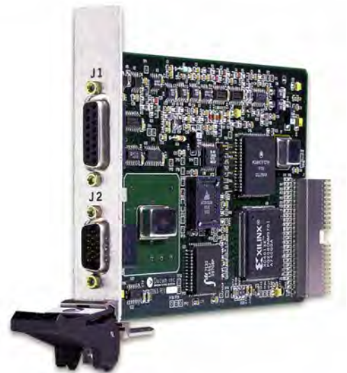
CPCI Time & Frequency Processor (shown with optional antenna/receiver, bc637CPCI)
