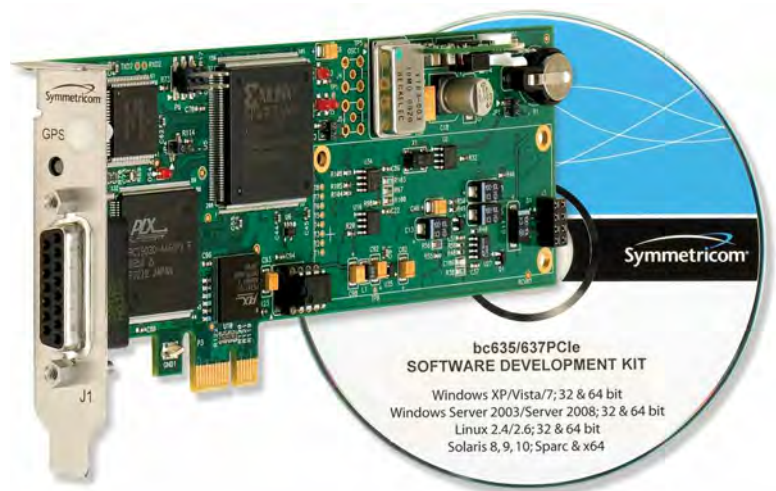
bc635PCIe Time & Frequency Processor & Included SDKs/Drivers
