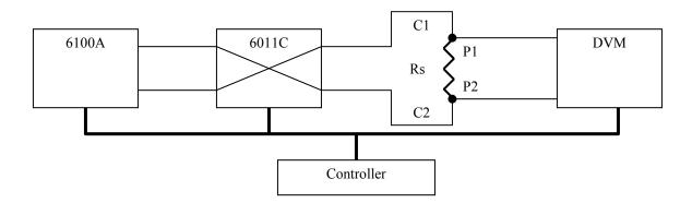
The 6011C Range Extender may also be used in conjunction with MI's Model 6010 Resistance Bridge and 6100A DC Power Supply. The Model 6010/6011C/6100A provides automated, accurate measurements from .0001 Ohm to 0.100 Ohm directly against a 1-Ohm primary standard automatically.
