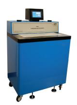
The 9400 comes standard with IEEE-488 and Serial RS232 Interface and can be controlled via M e a s u r e m e n t s I n t e r n a t i o n a l's resistance bridge operating software.
