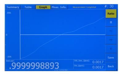
The graph screen displays a graphical representation of the individual measurement data plots.
