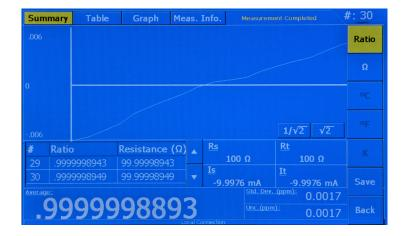
The Summary tab screen displays measurement parameters as well as graphical information for current measurement and can be viewed in ratio or Ohms at any time.
