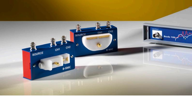
In combination with the Vector Network Analyzer Bode 100, the impedance adapters B-WIC and B-SMC are the perfect choice for **impedance measurements** of **passive electronic components**. The B-WIC is especially designed for through hole type components, while the B-SMC is the ideal adapter for all common passive surface mount devices.
