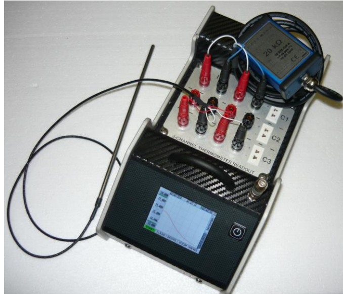
Figure 2: UT-ONE with reference resistor connected to channel C1
