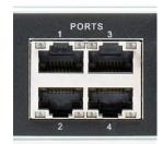
SyncServer S600 Series LAN Ports have hardware timestamping capability built-in ready to support PTP operations.
