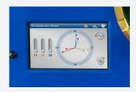
**Front Panel Display** The 4000 family now features a color touch screen display built into the test board front panel. This display provides information from the internal removable RX Reference Standard; including Energy Metrics, Vectors, Status, and more.
