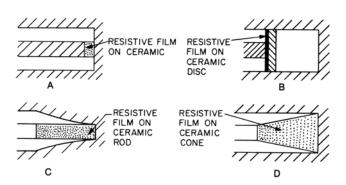
There are several ways in which a matched termination for a 50-ohm coaxial line may be realized. Some of these are shown below. Illustration A of the Figure shows
