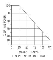
is calculated by using catalog specifications and a straight line graph. For instance the power rating of the Model 1430 attenuator is 100 watts at 25°C ambient and 10 watts at 125°C. Using linear graph paper, plot a straight line between these two points. This plot shows that the power rating at 75°C is approximately 56 Watts.
